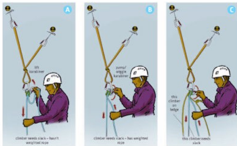
Figure 14.16 Methods of giving slack to second/s when belaying in guide mode (A) Climber hasn't weighted rope. Hold brake rope firmly, lift braking karabiner upwards while pulling slack through with other hand (B) Climber has weighted rope. Pump/wiggle braking karabiner up/down but keep tight grip on brake rope (C) Two climbers - one needs slack. Add back-up knot to brake rope of other climber and instruct to stay still. Use method shown in A or B to give slack
